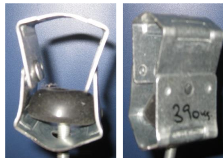
Failure load to traction of the TGOM 50
